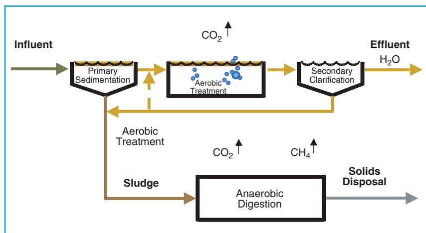
figure 2. The wastewater treatment process schematics.
